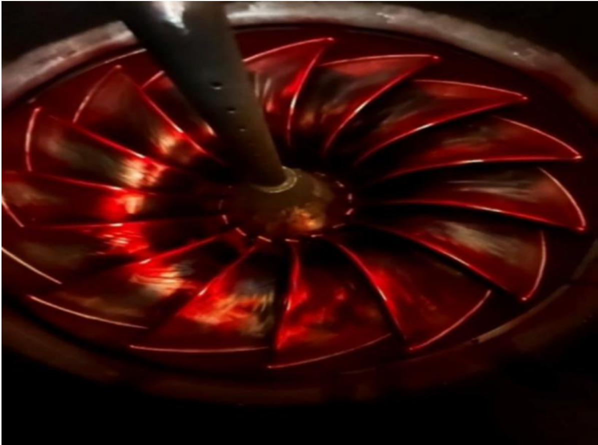
Unit #1 Runner after Dye Applied
