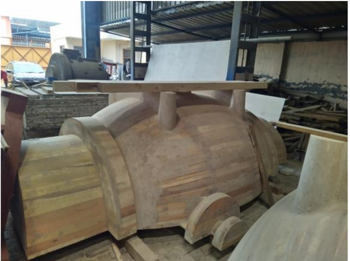
Plunger Valve Casting Mold
